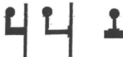
GRIPPABLE HANDRAIL DESIGNS: Grippable Area = 1 1/4" to 2" cross section
