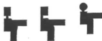
GRIPPABLE HANDRAIL DESIGNS: Grippable Area = 1 1/4" to 2" cross section
